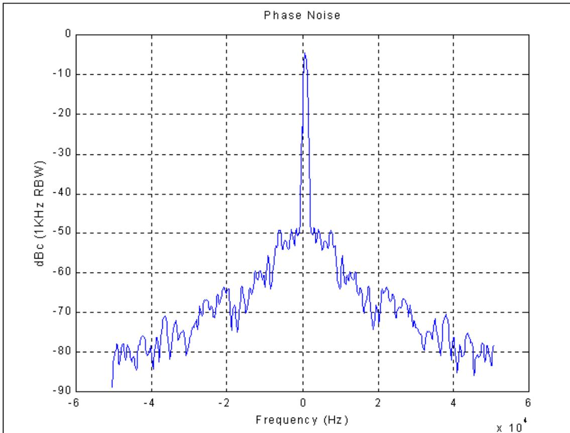
**Figure 1. Phase noise of test equipment**
