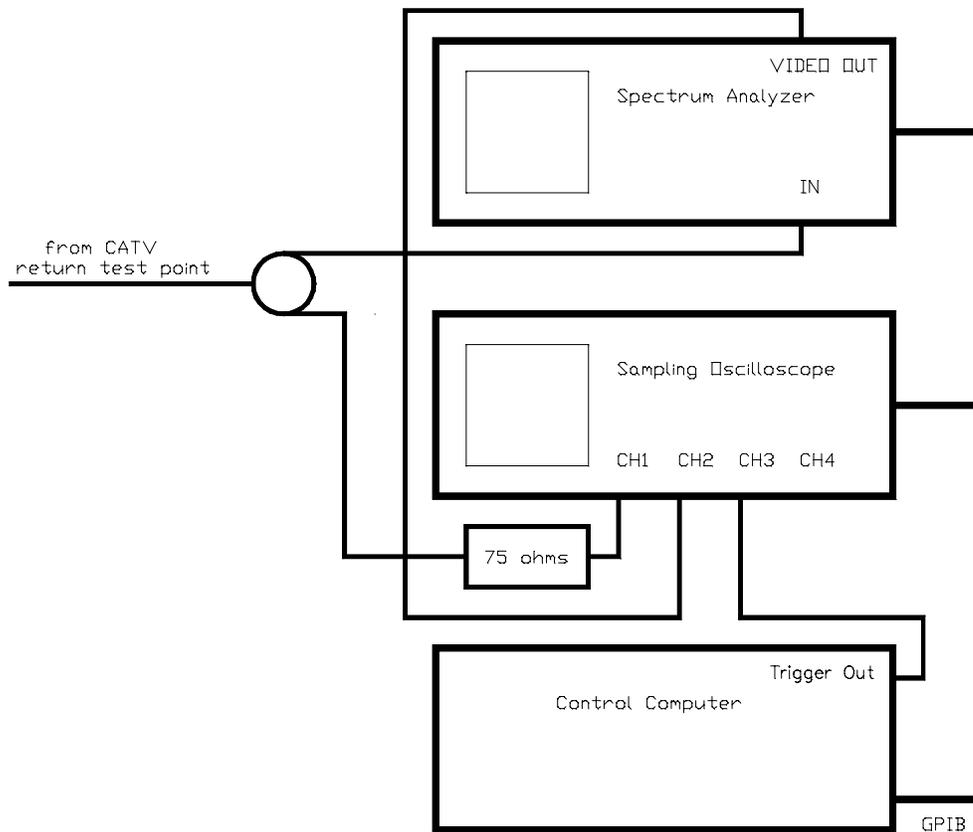
**Figure 1: Equipment setup**
