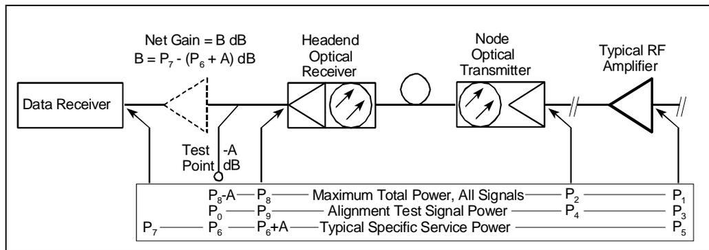
**Figure 2: Symbolic Diagram of Upstream Showing Level Reference Points**
