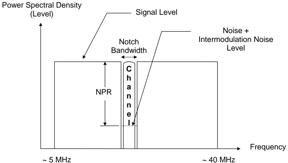
**Figure 1: Spectrum of Measurement Signal**
