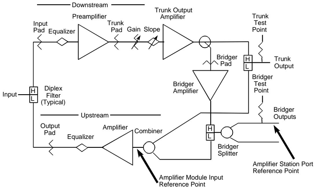
**Figure 1: Typical Amplifier Station Showing Reference Point Choices**
