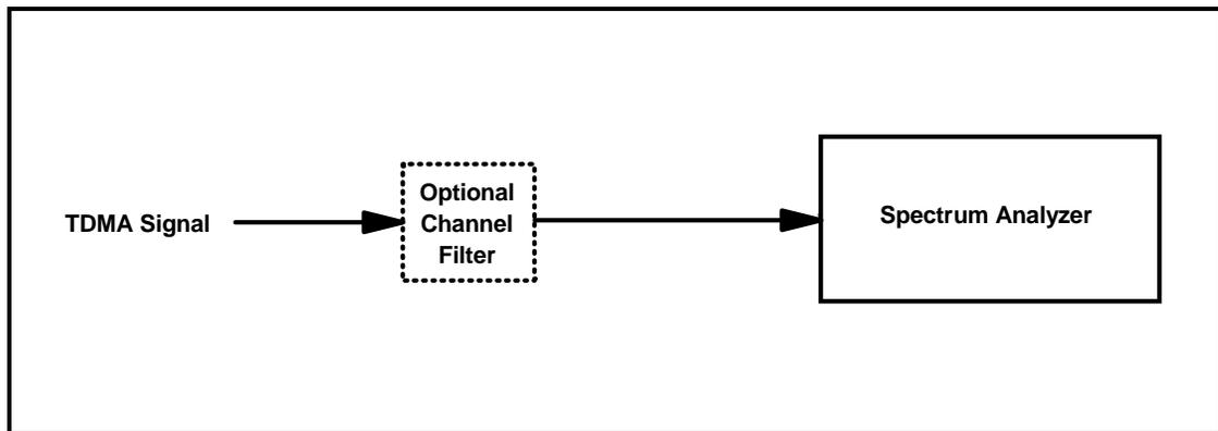
**Figure 1. Spectrum Analyzer Measurement Setup**
