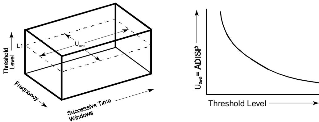
**Figure 2: Average Discrete Interfering Signal Probability vs Threshold Level**
