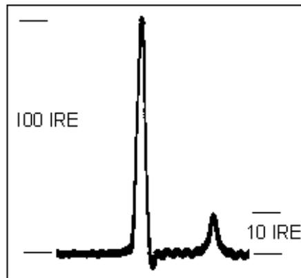
Figure 2. 2T pulse with - 20 dB reflection
