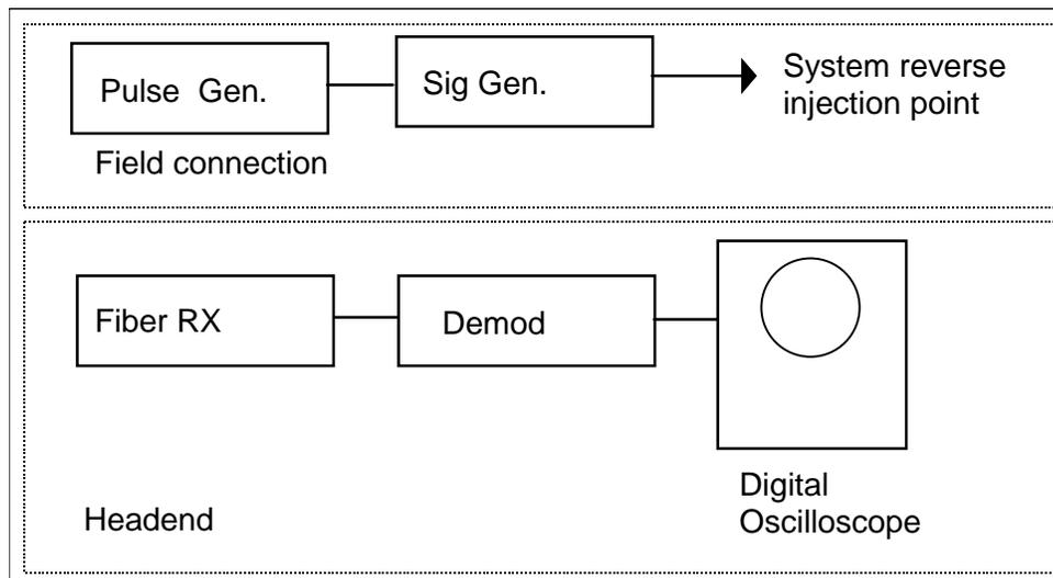
Figure 3. Equipment connection
