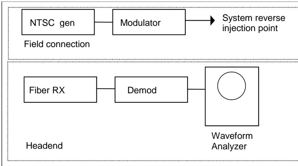
**Figure 1. Equipment Connection**
