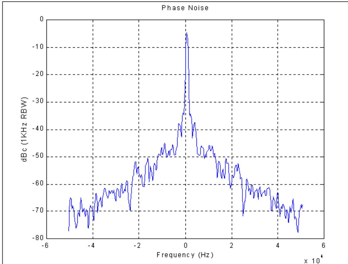
Figure 2. System phase noise
