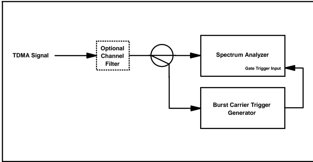
**Figure 2. Typical Gated Spectrum Analyzer Measurement Setup**
