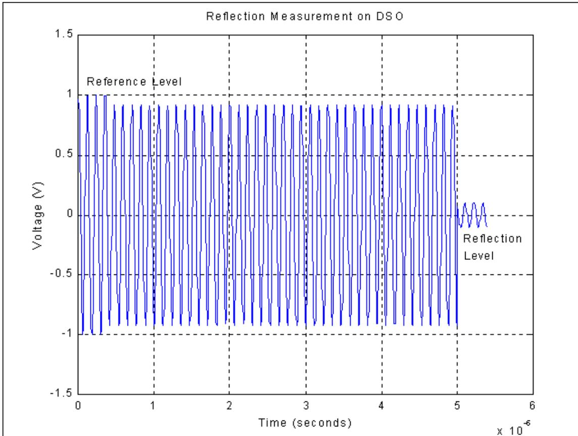
Figure 4. Example of -18 dB reflection
