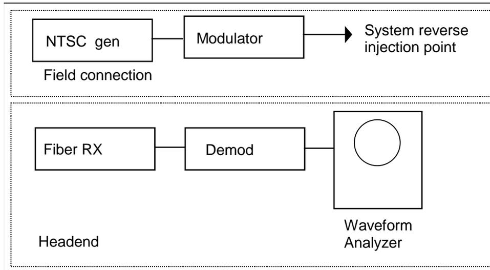
Figure 1. Equipment connection
