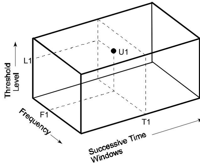
**Figure 1: Discrete Interfering Signal Probability (DISP) Data Base**
